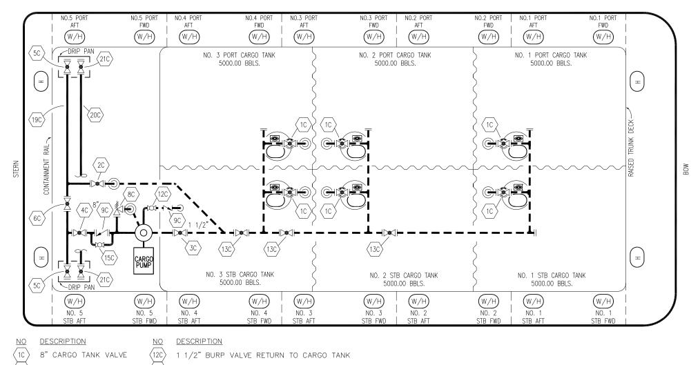
2C LOAD VALVE (13C) 8" CARGO PIPING BLOCK VALVE 3C MASTER SUCTION VALVE (15C) 1 1/2" BYPASS VALVE (AROUND CHECK VALVE) 4C 8" DISCHARGE VALVE (19C) 8" CARGO HEADER 5C 6C 8" HEADER VALVE (20C 8" DUMMY HEADER PIPING 8" SALVAGE VALVE 8" DUMMY HEADER VALVE KIRBY INLAND MARINE 8C ABOVE DECK PIPING 8" RELIEF VALVE CHECK VALVE BELOW DECK PIPING **CARGO DIAGRAM** 09/28/18 MRV OF ISSUED FOR APPROVAL BY CHK REVISION DESCRIPTION SCALE: NONE **HFL 404** 1 OF 3 PAGE:
